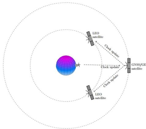
Time transfer using GNSS/GEO satellites
