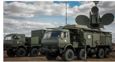
The Russian Krasukha-4 is designed to jam low-orbit signals, drones and missiles
