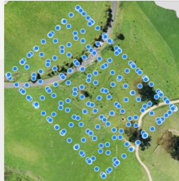
Grid plan was used to create a comprehensive 3D model and aerial map
