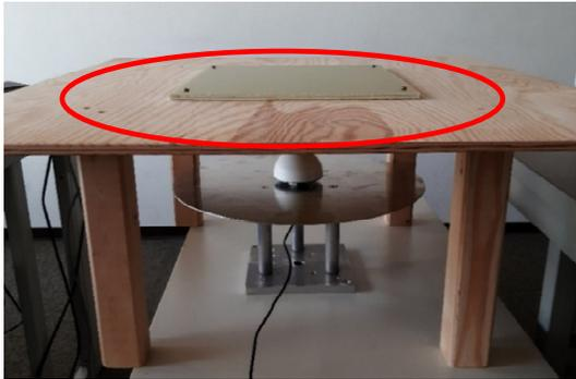
GNSS antenna under self-constructed cover plate using fiberglass-reinforced plastic (the same material as the train's roof)
