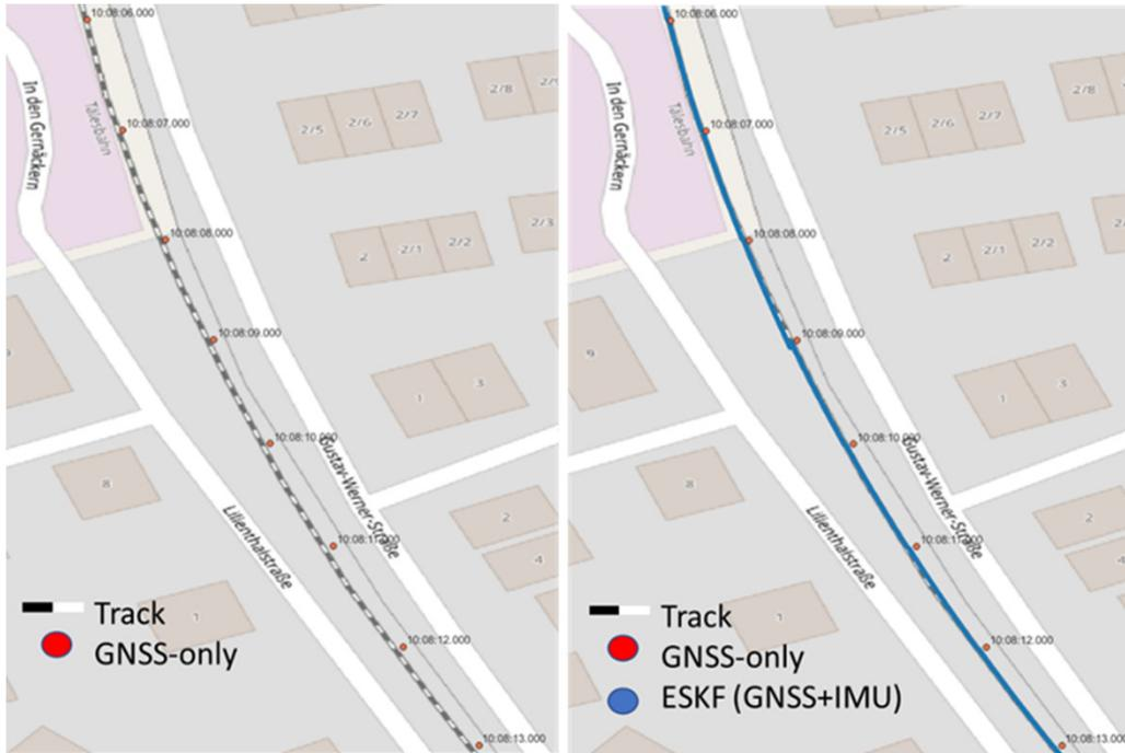
GNSS-only (float solutions) vs. ESKF (GNSS+ IMU) for one track section
