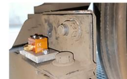
IMU on the bogie
