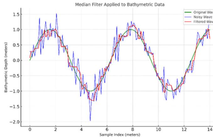
Figure 6: The illustration of median filter application in bathymetric data
