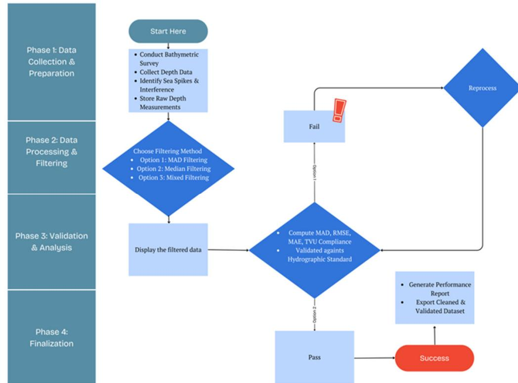
Figure 4: The flowchart of the system development SSFS
