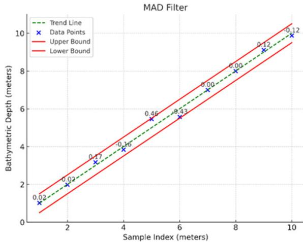
Figure 5: The illustration of MAD filter in outliers' detection
