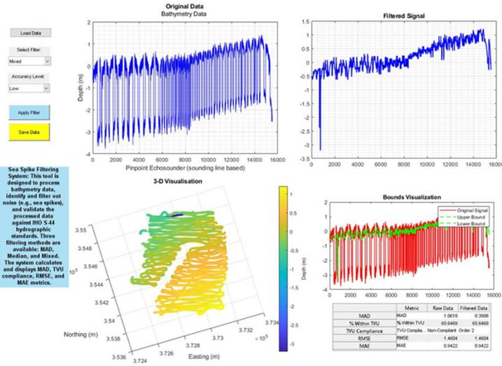
**Sea Spike Filtering System:** This tool is designed to process bathymetry data. Identify and filter out noise (e.g. sea spikes), and validate the processed data against IHO S-44 hydrographic standards. Three filtering methods are available: MAD, Median, and Mixed. The system calculates and displays MAD, TVU compliance, RMSE, and MAE metrics.
