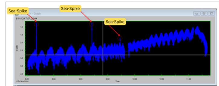
Figure 2: The bathymetry data that contained spikes shown in Hydropro Nav Edit
