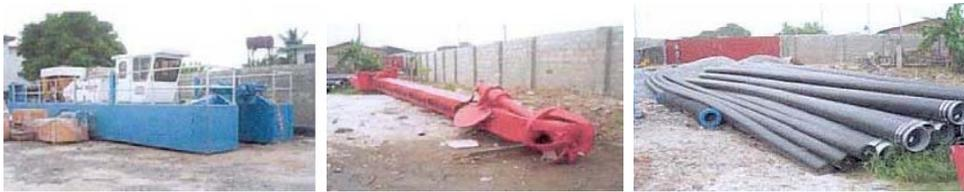
**Figure 4b:** A 12" x 10" elicott truckable cutterhead suction dredge powered by a 370 hp caterpillar diesel engine, with a 10m ladder and maximum digging depth of 6.1m. Included are 500 metres of 12 inch hdpe pipe with 300 metres of 8 inch hdpe floats.
